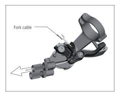
Fix the cable with the 2mm allen screw on the barrel adjuster on the fork crown with a tightening torque of 0.9Nm/ 8lb/in, cut the cable and secure it with a cable end-cap. Please refer for this action also to the manual of SRAM/RockShox attached to the bike.
