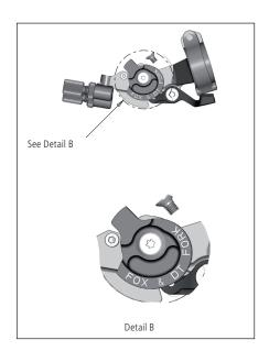
To assemble the cable please bring the lever into the Full (Travel) Mode
