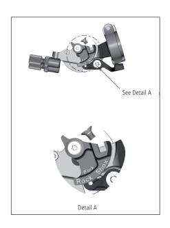
To assemble the cable please bring the lever into the All Travel Mode, push the cable into the lever-eyelet as shown on drawing below, push it through the pre-cut cable housing and fix it at the assembly unit on top of the right side of the fork crown.
