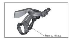
Change the modes by pushing the lever with your fingers frontward and release them by tapping the release button (one mode per push/release)
