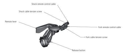
Regarding the installation and adjustment of the rear shock remote cable please follow the instructions of the different shox attached to your bike. Please note that the cable for the rear shock is ALWAYS the upper cable on the lever as shown in drawing below. There are 3 different versions for different rear shock models.
